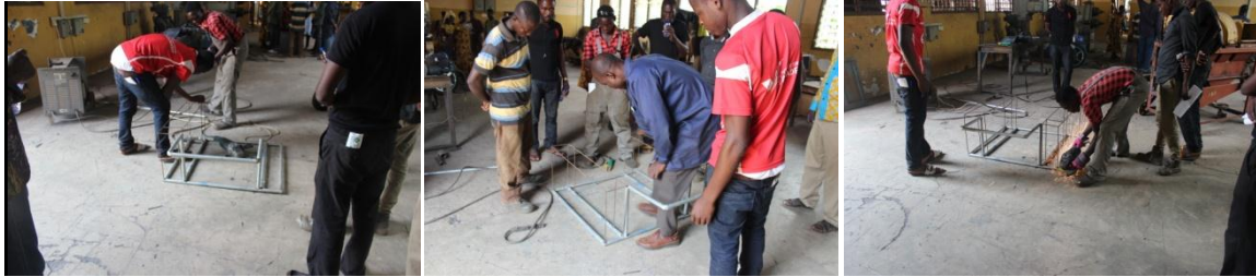
Figure 2: Farm Pull cart under various stages of fabrication by participants
