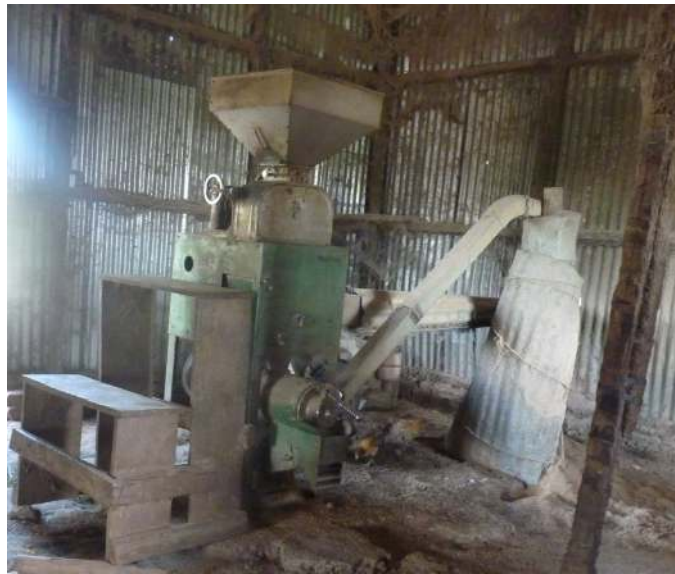
Figure 8. A typical one pass vertical rice milling machine with separate outlets for husks and bran
